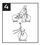
While sitting on the top tube of the frame firmly press down on top of the upper hook with downward force matching the arrows then close the clamp.
