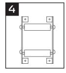
Repeat steps to install rollers with the 3 remaining button head bolts
