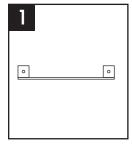
Insert M6 bolts into rubber feet. With side rail face up place one rubber foot/ bolt assembly through hole and secure with one nut
