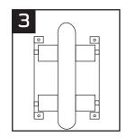
Place the rear wheel between the two rollers on the unit, making sure your rear wheel is parallel with the side rails of the unit
