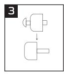
Locate the 4 rubber feet and 4 M6 bolts. Install M6 bolts from the under side of the rubber foot. The bolt will be sticking up from the flat side of the rubber foot. Firmly press in M6 button head bolt into each of the rubber feet.
