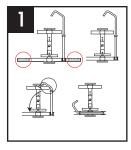
With unit assembled, stand over the unit with your heels in the area circled in red. Lower the Upper hook until it is fully inserted in the lower vertical upright. Next grab the Upper hook in area circled in black and rotate counter clockwise until the vertical upright is parallel with the lower base.
