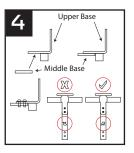
Grab the upper base and middle base. Place middle base under the wheel support and match the two threaded holes in the middle base with the two holes in the bracket. Ensure that the "R" of facing in the correct orientation. Insert M6 bolt and tighten till snug.
