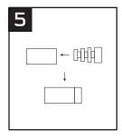
Locate 4 square plugs and press into the square opening on the left and right side of the base
