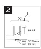
Locate U brace, 3/8 bolt, 3/8 washer, and 3/8 nut. Insert 3/8 bolt through U brace then install into the base. Flip over the base and place washer on bolt then screw on 3/8 bolt. Use a 14mm wrench to tighten till snug
