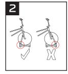
Double check to verify that the Roller Stand is in the correct orientation. The "U" brace, Lower base, Lower Vertical Upright, and Upper hook should be behind the front wheel.
