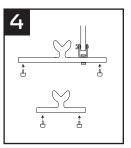
Install the 4 rubber feet to the under side of the base with M4 Allen key
