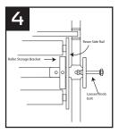
To remove Rexer Rollers loosen Knob bolt until there is enough room.
