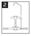
Grab upper hook and insert into the lower vertical upright where the seat clamp is attached.
