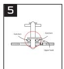
Place upper hook in the area in front of the fork and wheel. Upper hook should be touching both the left and right arms of the fork arms and front wheel.
