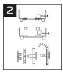
Remove the 4 x M6 bolts from the middle, upper, and lower base. Place hardware in a secure place. The unit is now ready for travel.
