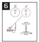
Using the longest M6 bolt out of the 8, place the roller bracket above the lowest hole on top of the bracket. Install M6 bolts and tighten till snug.
