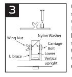
Grab the carriage bolt, wing nut, 2 white nylon washers, and lower vertical upright with seat clamp installed. Locate end with two holes, this side will be installed into U brace. Place white nylon washers in-between the inside of the U brace and the lower vertical upright. Install wing nut on the outside of the U brace, tighten till snug.
