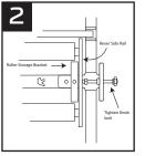
Tighten the Knob bolt until there is sufficient pressure against the outside face of the side rail on the Rexer rollers.
